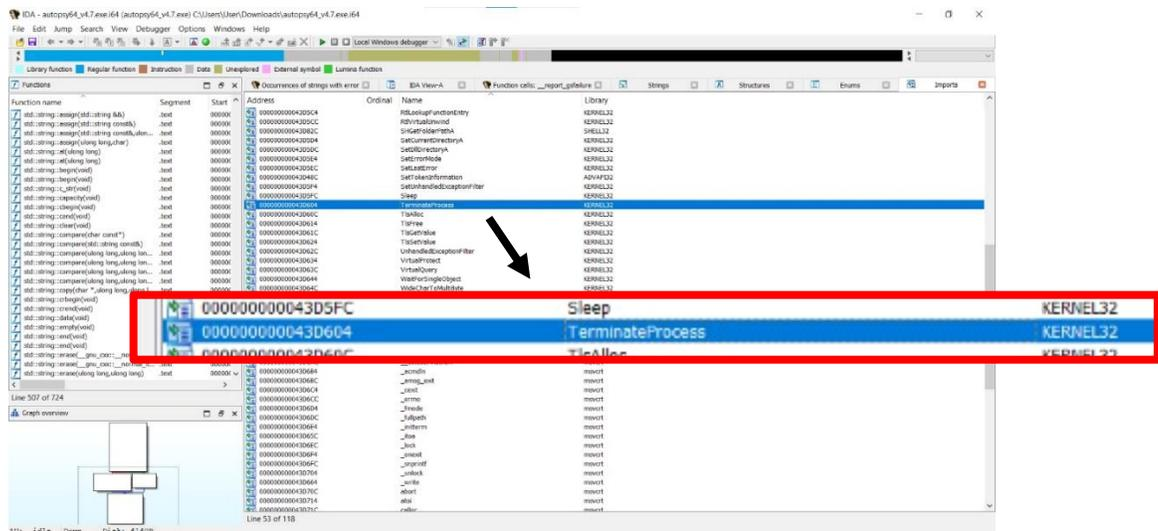
Fig 4. TerminateProcess is being imported from KERNEL32
