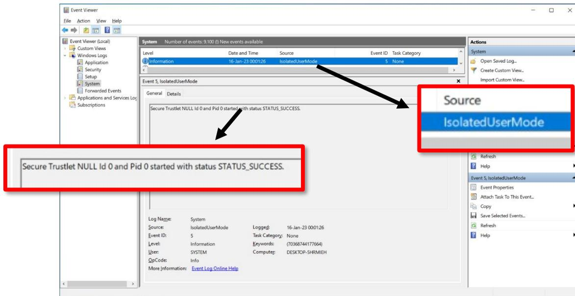
Fig 8. User successfully entering isolated user mode
